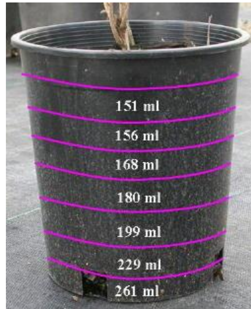
The volume of water held at each level of the container is listed. Water is not distributed evenly; the container bottom is saturated while the top is drier.
