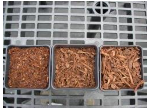
Bark particle size influences media physical properties. As particle size increases from left to right, so does total porosity.
